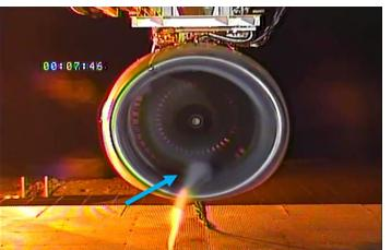
Eventhough ground vortices can be simulated and analyzed with CFD tools, **validation** of such studies is **challenging**: deploying the necessary instrumentation tools on an engine test survey is incompatible with the **integration constraints** (stress, intrusiveness, cost)
