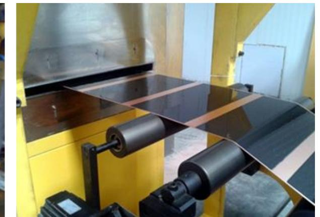
Coating (max. 5 m/min, max. 40 cm width) *Double sided gap coater*
