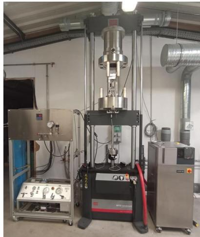
High pressure hydrogen testing
